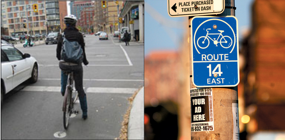
Left: Cyclist on bicycle actuated dots that activate traffic signal. (City of Toronto)
